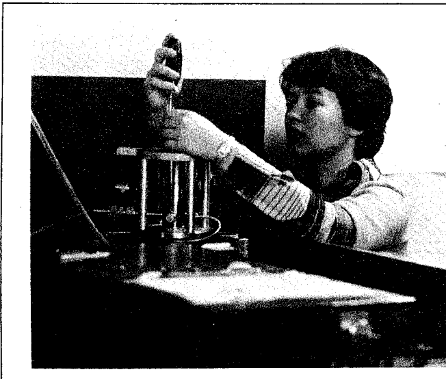
Shown here is Stanford graduate student Sally Hunter. Sally's work is supervised by Professor Bienenstock. She grew up with the SSRP facility, learning the technique of Extended X-ray Absorption Fine Structure (EXAFS) experiments in the process. She is shown here working on a liquid-nitrogen dewar system used in low-temperature EXAFS studies. She expects to receive the Ph.D. in April of this year, after which she will join the SSRP staff.
