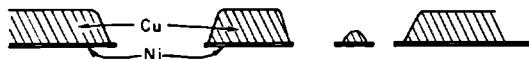
Figure 22-5 Cross section of a target showing how the apertures are formed by the 0.002-in. thick nickel plating on 0.02-in. thick copper sheets. Where the holes are small and closely spaced, all the copper was often etched away.
