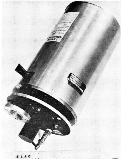
Figure 9-8b Litton sub-booster klystron.
