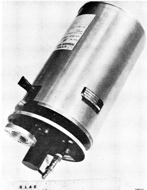
Figure 9-8b Litton sub-booster klystron.
